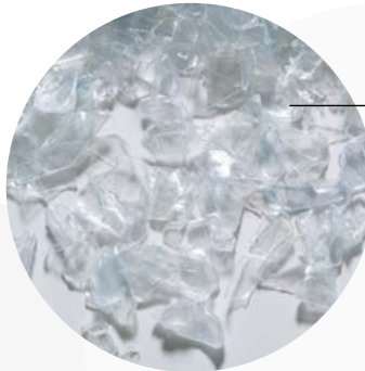
Bottle flakes after plastic washing system
