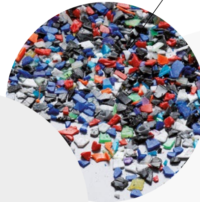
PP flakes for injection molded parts
